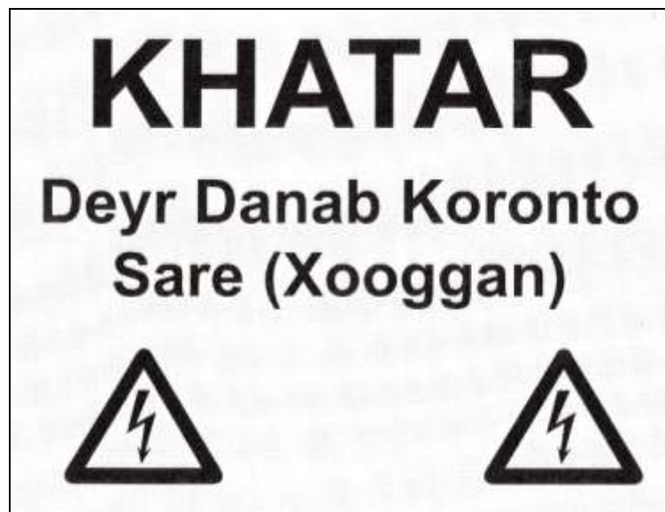
Example of a warning sign in Somali, which states – DANGER HIGH VOLTAGE ELECTRIC BARRIER
